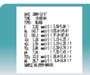
High-speed thermal printer, printing all the sample data, calculating data and reference ranges.
